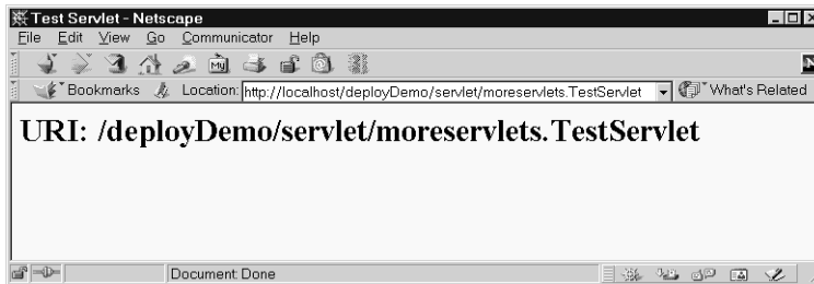
Figure 5-7 Successful attempt to invoke the TestServlet servlet by means of the default URL. The invoker servlet is enabled.
