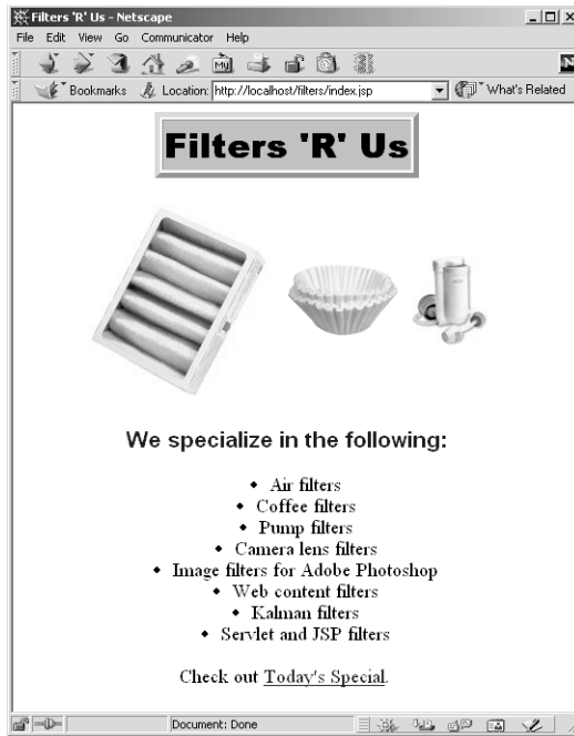
Figure 9-1 Home page for filter company. After the page is deployed on an external server and the reporting filter is attached, each client access results in a printout akin to “purchasing.sun.com tried to access http://www.filtersrus.com/filters/index.jsp on Fri Oct 26 13:19:14 EDT 2001.”
