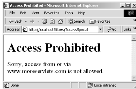
Figure 9-6 You cannot successfully follow the link from the page of Figure 9-5. The BannedAccessFilter prohibits access from www.moreservlets.com (an unscrupulous competitor to filtersRus.com ).
