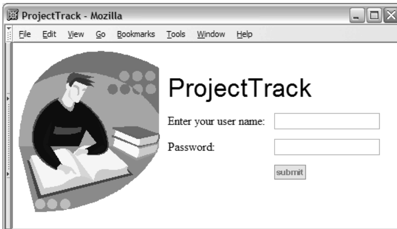
Figure 8.5 The Login page with an image for a button, JavaScript for a rollover, and CSS for formatting.
